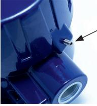
Always tighten the locking screw to prevent unintended opening of the head with flameproof enclosure.
